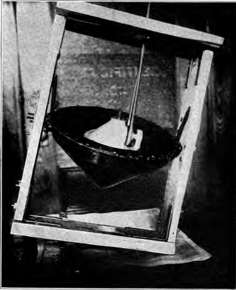
Fig. 24. Beach Gyroscopic Stabiliser
